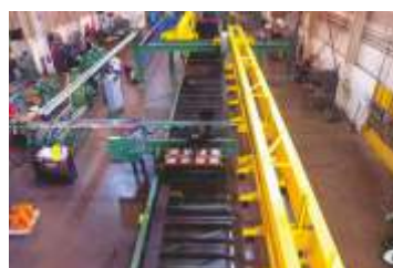
Welding by pull through machine
